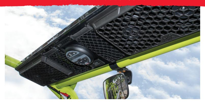
When you are looking for the performance of a bigger sound system in a low-profile chassis, then our overhead sound bars are a great option. With three different sizes available, the sound bars can adapt to most roll cage widths with ease and fit up to a 2" tubular diameter.
