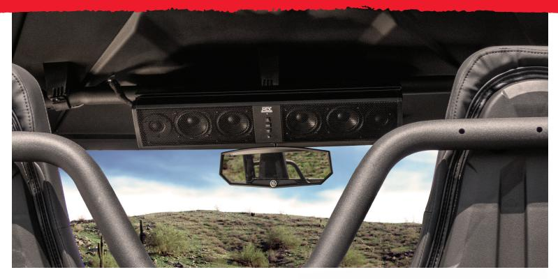
Our universal 6-speaker sound bars are a great choice when an overhead design isn't practical. With their multi-directional mounting system, they can be mounted almost anywhere on the vehicles roll cage. The internally amplified speaker system is available with an AUX input for music connection, or you can upgrade for added Bluetooth connectivity.
