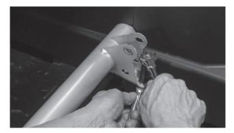
Step 7 - Remove the cable clamp from the brake line.
