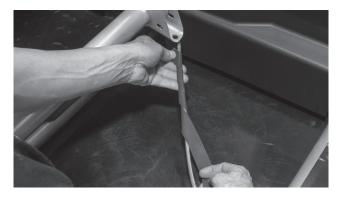
Step 9 - Tilt the front of the enclosure down and slide it under the forward crossbar as you set it in place onto the floor of the vehicle tucking the brake line into the pre-molded slot in the bottom of the enclosure.
