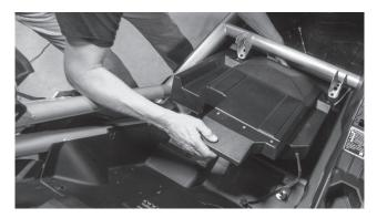
Step 10 - Taking the long bar bracket included, align the slotted holes with the threaded insets on the top rear of the enclosure. The two large holes at either end should slide over the threaded seat mounting posts.
