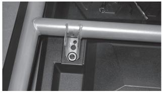
Step 13 - Once all fasteners are in place, tighten to secure the enclosure.
