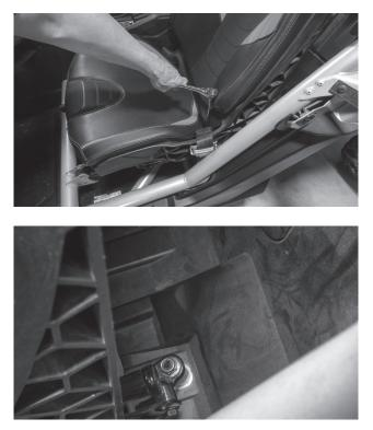
Step 4 - With the seat free, disconnect the seat belt sensor and speed sensor cables from the seat assembly.
