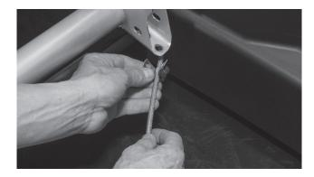
Step 8 - Wrap the brake line with the strip of adhesive backed foam tape included in the box. **Note:** This step is to prevent the brake line from rattling against the enclosure under high bass output and any chaffing due to movement of the brake line while the vehicle is in motion.
