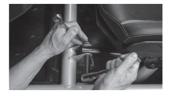
Step 3 - Access the rear 18mm nuts using a socket with extension either by aligning the holes in the seat base over the nuts or by sliding the seat fully forward and reaching behind.
