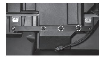
Step 12 - Align the threaded inserts at the front corners of the enclosure with the holes in the bottom of the seat brackets and insert two (2) T-40 Torx screws.
