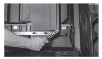
Step 14 - Route the subwoofer cable to the desired connection point. **Note:** If installing as part of a kit, the subwoofer plug will connect to the main harness supplied. If not installing as part of a kit, the plug will need to be removed and additional speaker wire added.
