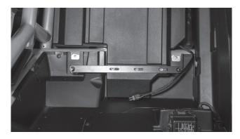
Step 11 - Loosely install three (3) T-40 Torx screws into the bracket.
