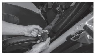
Step 2 - Remove two (2) 13mm bolts and nuts at the front of the seat frame.
