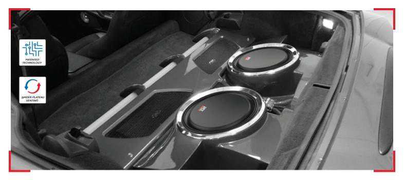
35 Series shallow mount subwoofers offer both the convenience of a shallow mount design with the awesome low frequency bass output that MTX has built its reputation on over our 40 years in the car audio industry. The 35 Series shallow subwoofers are only 3.375" deep, are optimized for sealed enclosures, and require as little as 0.6 cu ft of air space to function.
